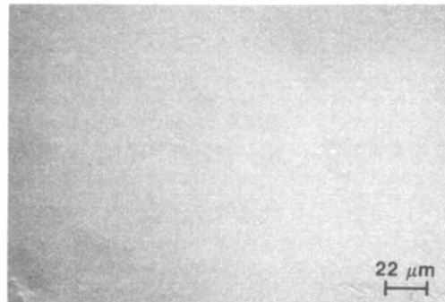
Fig. 16. SEM micrograph of the surface morphology of a Ti/Ni/AuSn sample after reflow at 320 °C for 60 s.
